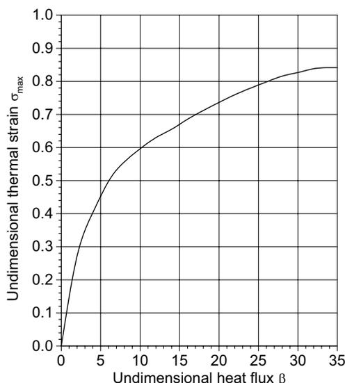
*Fig. 1. The dependence of u dimensional thermal tensions of  $\sigma_{max}$  from the undimensional heat stream of  $\beta$*
