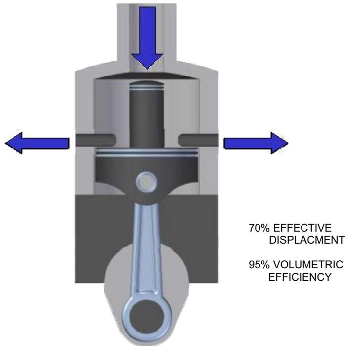
*Fig. 14. Compound Engine System with the cold piston centre section*
