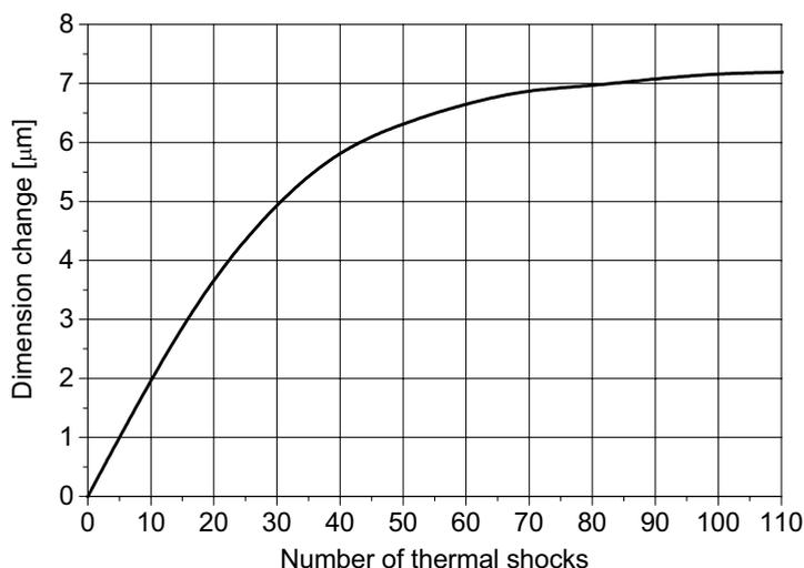
*Fig. 9. The example of the influence of the thermal shocks number on the deformation of the piston sample*
