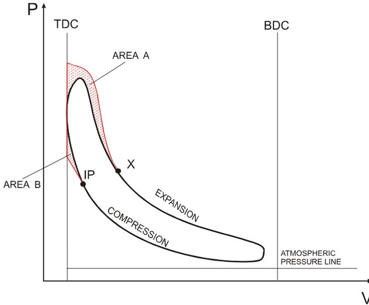
Fig. 10. Pressure changes in the piston stop cycle, Compound Engine System
