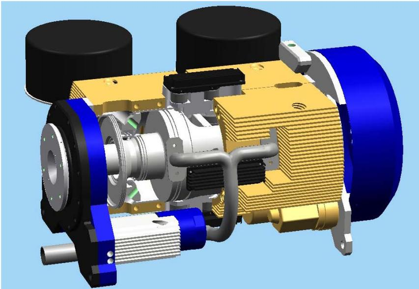
Fig. 11. Compound Engine with piston stop configuration (swashplate)
